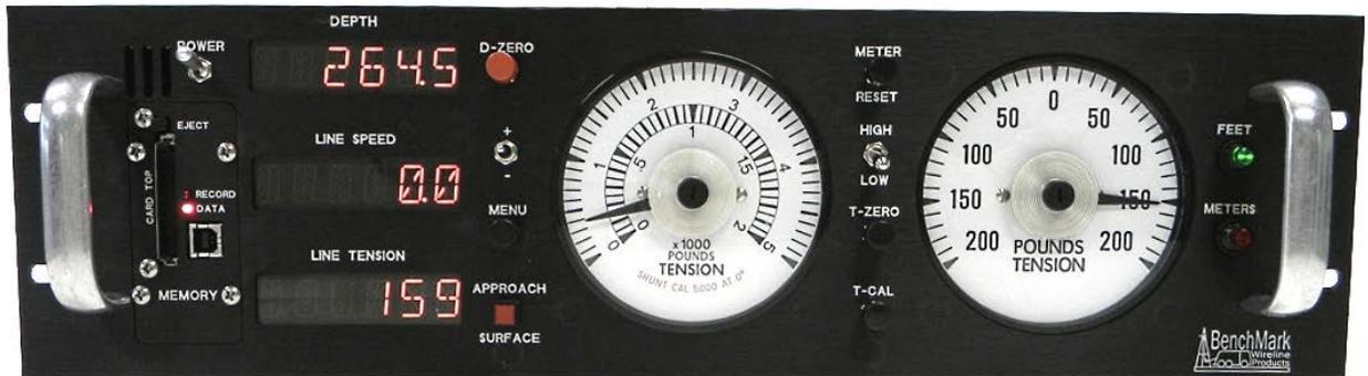
This panel is designed to acquire and display depth and tension from a wireline winch unit. The panel uses a menu system to set and make adjustments to the data as necessary.
